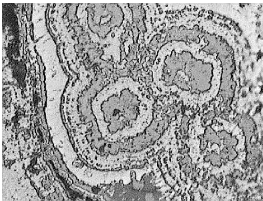
Figure 2. Compact pyrite ore, with rhythmic colloform textures cemented by galena (gray) and sphalerite (dark gray).
